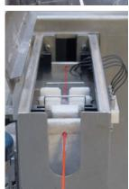
UMAC® WALLMASTER systems from ZUMBACH allow in-line measurements, data acquisition and control during the extrusion of a wide range of products, like tubing, pipe, hoses and cables. Cutting edge digital technology (DSP) opens up measuring solutions for each process and product:
